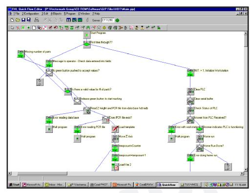
Quickflow provides an easy to use visual programming system for controlling the flow of products through your marking area. Unique part identification yields the ultimate in quality control and product traceability.
